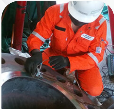
Phased Array Ultrasonic Testing (PAUT)
